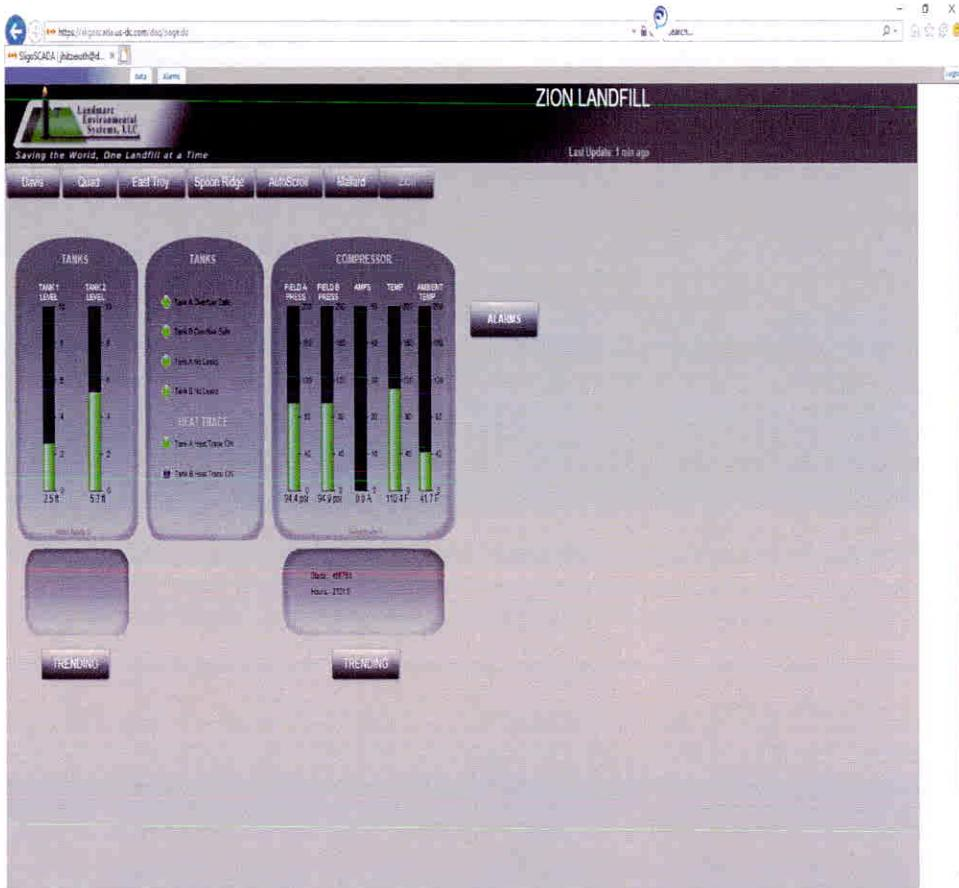
The Site 1A tank is "Tank 1". The "Tank A Overflow Safe" indicator is tripped based on a sensor monitoring the overflow pipe from the tank to the secondary containment. The Tank A "No Leaks" indicator provides an alert based on a sensor located in between the dual tank wall containment if the interior wall is breached and liquid is detected in the space between the primary and secondary tank walls.
